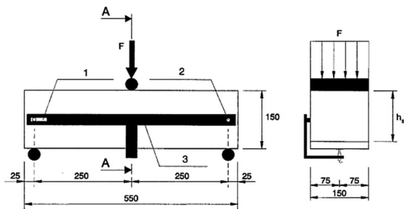
Figure 2: Three point bending test with notch according to EN 14 651
