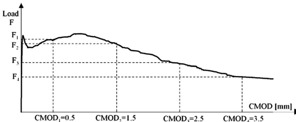
Figure 3: result of Results of the beam test – Load vs crack mouth opening displacement (CMOD)
