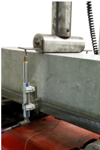
Figure 4. EN 14651 relationship between CMOD and midspan displacement \delta .
